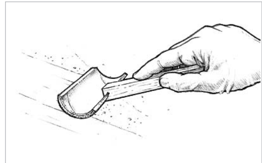
Figure 5-24 Tip off the fresh coat of epoxy with the grain, using a foam roller brush to remove bubbles and roller marks.
