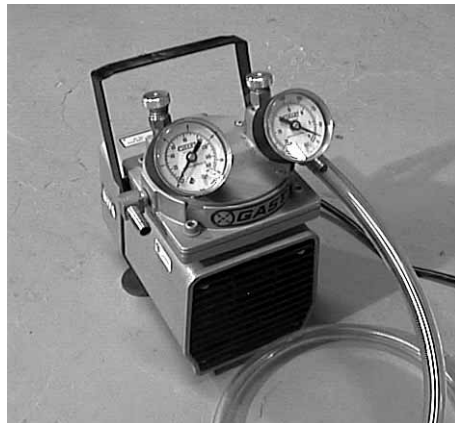
Figure 2-3 A Gast Model 07061-40, 1/8 hp diaphragm pump. This pump displaces 1.2 CFM and will achieve a maximum vacuum pressure of 24.0" Hg. It is a practical pump for small projects.
