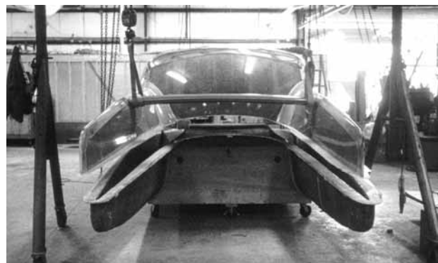
Figure 4-7 A finished laminated part (deck/cabin), suspended over the bottom (hull) mold. The mold also serves as a jig to hold the laminated hull in place while interior components and the laminated deck are bonded in place.
