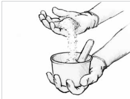
Figure 5-7 Blend in small handfuls or scoops of the appropriate filler until the desired consistency is reached.
